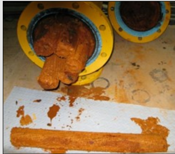
The wells became contaminated with iron and suspended solids which plugged the system's heat exchangers and pipes.
